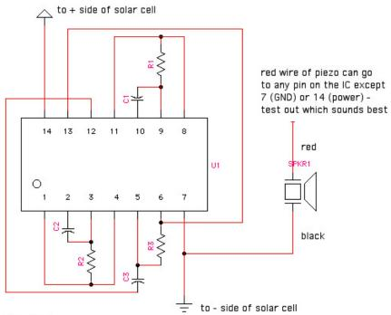
R1, 2, 3 - resistors,  $100\Omega$  - 100k C1, 2, 3 - capacitors,  $1\mu\text{F}$  -  $47\mu\text{F}$  U1 - IC 75HC14 SPKR1 - piezo speaker, Radioshack 273-060 power from solar cell (around 3V)
