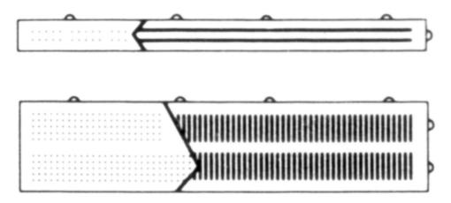
The bus rows, usually 2 on each side, are reserved for positive power and ground. The holes in the center columns are for components. The divider between the columns will be very useful when we start working with ICs (Integrated Circuits). It assures that each pin of the IC has its own column for other parts to be connected to it.
