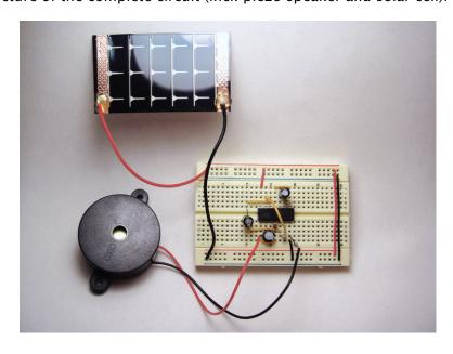
If you do not hear a chirping right away, go outside and expose the solar cell to the sun or hold it very close to an incandescent light bulb. If you still do not hear anything you might have the wrong type of piezo (not suitable for 3V output), the wrong type of solar cell (cannot produce at least 2.5V) or you have made a mistake in your circuit. In this case, go back to page 4 and follow all the connections (sometimes checking the ones you have followed with a pencil is helpful).
