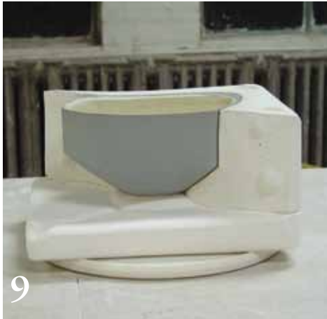
9 Cast bowl, dried and ready to remove from the mold.
