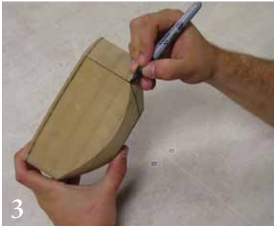
3 Finish shaping the prototype on a band saw and draw seam lines.
