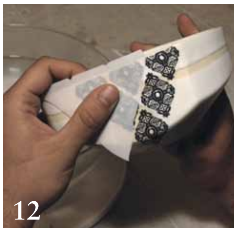
12 Applying the decal onto the fired bowl by sliding away the paper backing.
