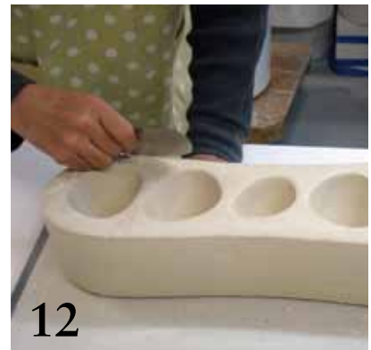
12 Gently scrape away excess slip flush to the surface.
