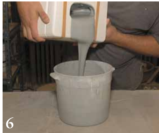
6 Drain the excess colored casting slip from the plaster mold.
