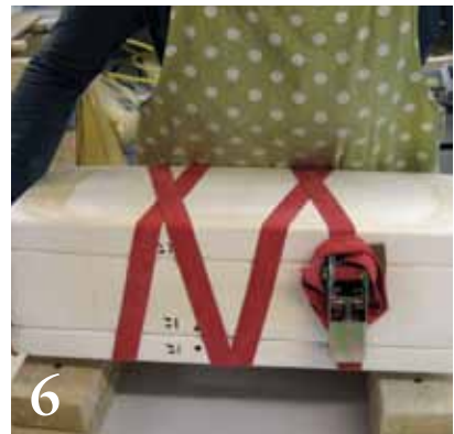
6 Flip the mold to allow slip to fill pour holes and finalize the casting.
