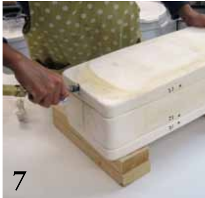
7 Use compressed air to release the casting from the plaster mold.
