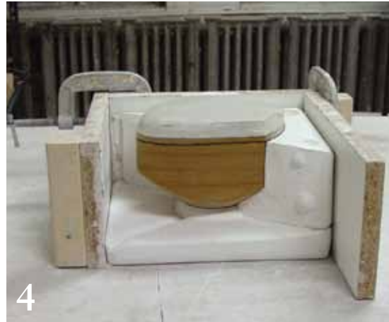
4 Add a clay slab to the sealed prototype to create a pouring gate or slip reservoir.
