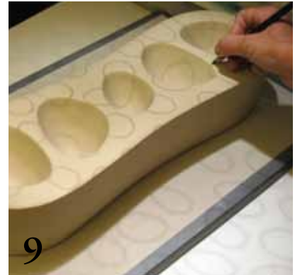
9 Trace a pattern on the surface using prism projector.
