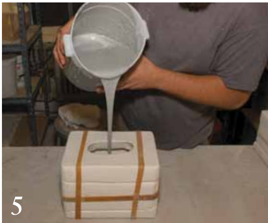
5 Pour colored casting slip into the plaster mold first.
