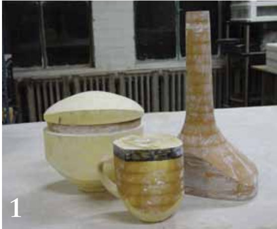
1 Finished wooden prototypes of various vessels sealed with polyurethane.
