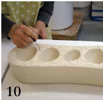
10 Carve the traced lines with a needle tool.
